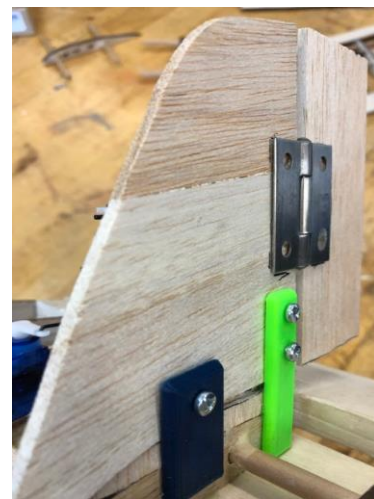
Figure 10: Final Rudder Design
