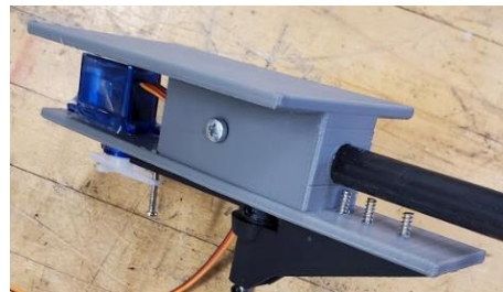
Figure 14: Final Design for Empennage Connection
